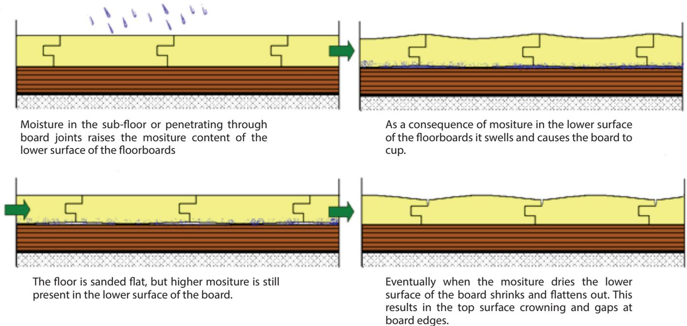
Figure 1 - The process of crowning
