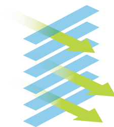
LOUVRE WINDOW 90% Fresh Air (Regardless of wind direction)
