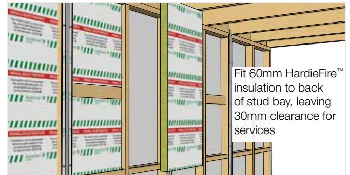
FIGURE 20 HARDIEFIRE™ INSTALLATION
