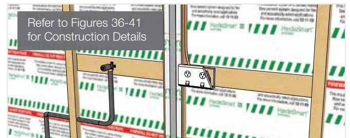
FIGURE 21 INSTALLATION OF SERVICES
