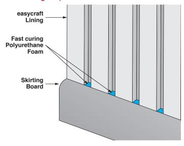
Use fast curing Polyurethane foam (Sika Boom AP) to fill gaps found between Easycraft Silhouette profile and rear side of your skirting board. (then cut, sand and paint)
