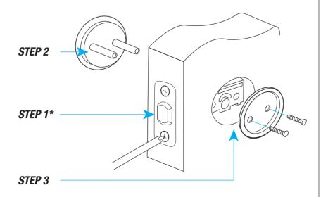
\*Proper installation allows the "thumb pull" to open from bottom, as shown.
