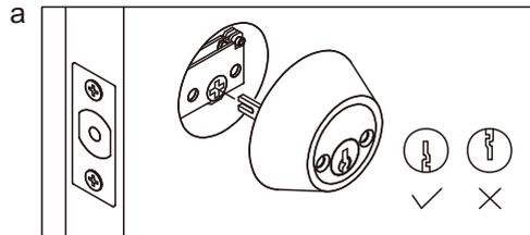
b. The interior tailpiece is inserted into the exterior blade.
