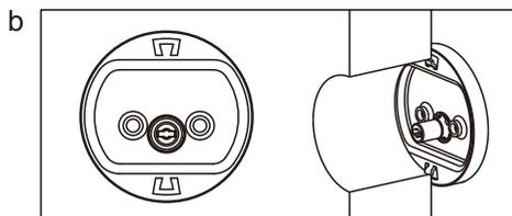
c. Insert machine screws through holes engaging holes in cylinder and tighten firmly.
