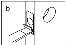
b. Chisel 5/32" (4mm) deep or until face plate is flush with the door edge.
