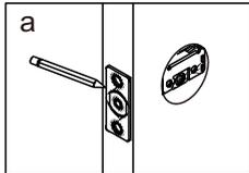
a. Insert latch in hole and keep it parallel to door face. Mark outline of face plate and remove latch.
