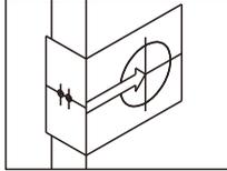
Backset is a distance from door edge to centre of hole on door face. Some locks are supplied with adjustable latch which can fit 2-3/8" (60mm) or 2-3/4" (70mm) backset. Just follow the steps shown below to change backset.
