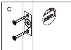
c. Insert latch and tighten screw.
