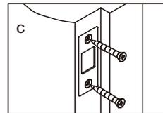
c. Install strike and tighten screws.
