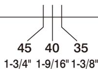
Mark 1" (25.4mm) hole at center of door edge.
