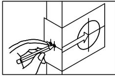
Select 2-3/8" or 2-3/4" (60mm or 70mm) backset as desired and mark centre of hole on door face.
