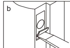
b. Measure one half of door thickness from door stop and vertically mark center line of strike. Drill 1" (25.4mm) hole, 1" (25.4mm) deep at intersection of horizontal and vertical line of strike. Mark outline using strike plate and chisel 1/16" (1.6mm) deep for strike.
