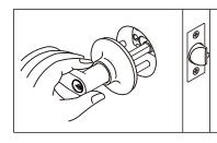
Insert spindle through latch.
